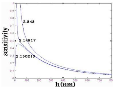
**Figure 5: Sensitivity with the Film Thickness for  $n_f = 2$ ,  $\epsilon_s = 2.131917$ ,  $\epsilon_c = 2.130213$ ,  $\epsilon_c = 2.14917$ ,  $\epsilon_c = 2.343$**
