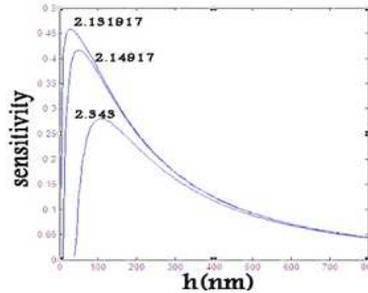
**Figure 1: Sensitivity with the Film Thickness for  $n_f = 2$ ,  $\epsilon_c = 2.13$ ,  $\epsilon_s = 2.14917$ ,  $\epsilon_s = 2.131917$ ,  $\epsilon_s = 2.343$**
