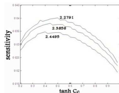
**Figure 6: Sensitivity with the Film Thickness for  $\epsilon_s = 2.343$ ,  $\epsilon_c = 2.2791$ ,  $\epsilon_c = 2.3856$ ,  $\epsilon_c = 2.4495$ ,  $h = 0.1 \mu\text{m}$**
