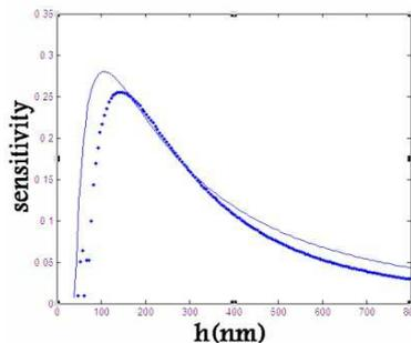
**Figure 3: Sensitivity with the Film Thickness for  $n_f = 2$ ,  $\epsilon_c = 2.13$ ,  $\epsilon_s = 2.343$  for the Proposed Nonlinear Sensor (Solid Line) and a Linear Sensor (Dotted Line)**
