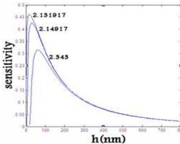
**Figure 2: Sensitivity with the Film Thickness for  $n_f = 2.34949$ ,  $\epsilon_c = 2.13$ ,  $\epsilon_s = 2.14917$ ,  $\epsilon_s = 2.131917$ ,  $\epsilon_s = 2.343$**
