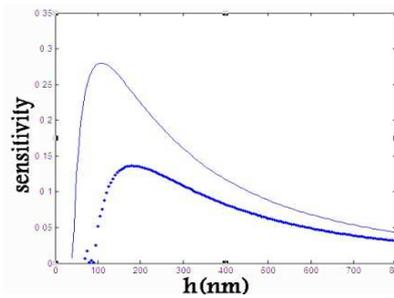
**Figure 4: Sensitivity with the Film Thickness for  $n_f = 2$ ,  $\epsilon_c = 2.13$ ,  $\epsilon_s = 2/343$  for the Proposed Nonlinear Sensor (Solid Line) and  $n_f = 2$ ,  $\epsilon_c = 1.8$ ,  $\epsilon_s = 2.6$  for the Previous Research Works (Dotted Line)**
